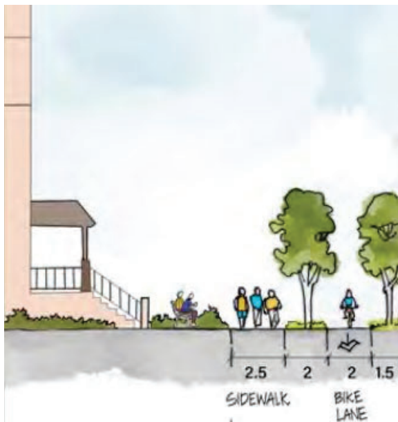
Figure 3: Example of a cross section with active transportation and public realm elements behind the curb
